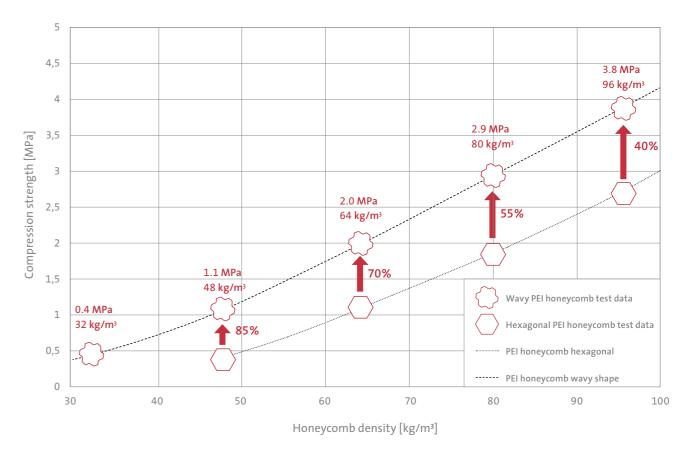
ThermHex<sup>wavy</sup> PEI honeycomb core is a continuously produced thermoplastic honeycomb core with exceptional fire resistance and temperature stability.
